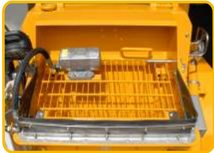
Specially designed hopper with agitator and vibrator grill for shotcrete operation with steel / polymer fibres.
